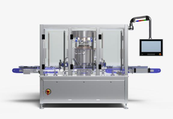
The Aptus is a fully automated, servo driven, constant motion. rotary crimper. Ideal for mid to large production runs of time sensitive products such as lyophilized vaccines, the Genesis Aptus is capable of sealing both large and small parenteral vials at up to 300 vials per minute.
