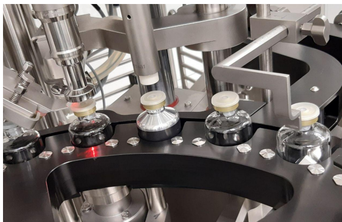
Figure 2. Seal Tightness drone in the capping process.
